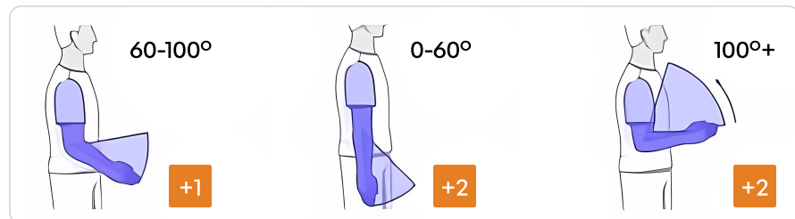
Figure 4 Computation of the elbow angle and the calculation of the REBA score. 3
